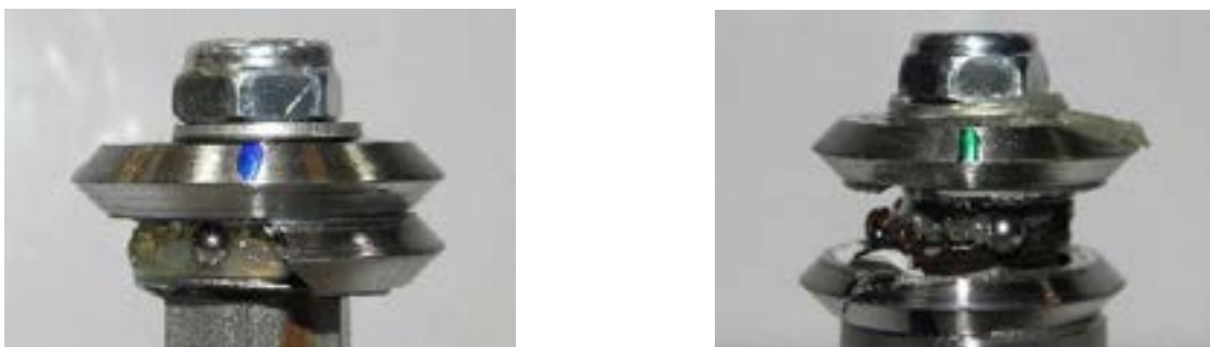
FIGURE 6: Shown here are two examples of catastrophic failure exhibited by competitor guide wheels. With these components, shards and ball bearings have the potential to fly off and hurt bystanders, damage other machine components, or contaminate material the equipment is responsible for processing.
