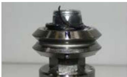
FIGURE 7: This is a Bishop-Wisecarver guide wheel exhibiting a condition that's typical for this product line's mode of end-of-life failure. No shards or fractures are present — and the component is essentially intact.
