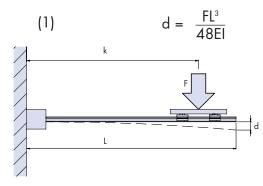
The deflection of a Slide beam acting as a cantilever and using a Long Flange Clamp (as shown opposite), will be a maximum at the free end when the load is at the outermost extremity of its stroke. This maximum deflection is given by the following equation:
