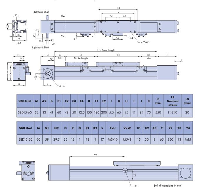
Re-lubrication of the ball guide carriage block is via an access point in the side of the beam (see above), which is closed off with a threaded plug. The lubrication interval depends on the length of stroke, speed and duty. For further details regarding lubrication procedures please contact Bishop-Wisecarver's technical department.
