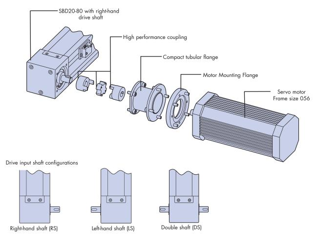
The hollow shafted arrangement may offer a more compact and lower cost means of retro-fitting a motor and/or gearbox onto an SBD. For more information, please contact Bishop-Wisecarver.
