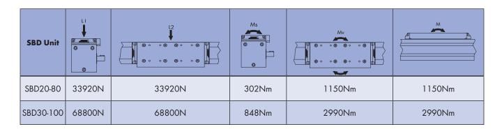
The table below includes the parameters necessary to calculate the performance and duty of an SBD system.
