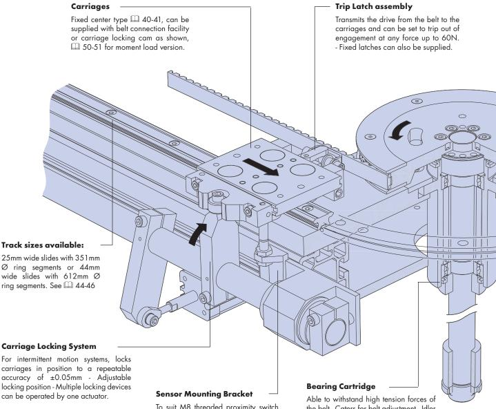
To suit M8 threaded proximity switch - Detects carriage position for control and safety purposes. the belt - Caters for belt adjustment - Idler type or, extended shaft type available for attaching the drive - Sealed bearings lubricated for life.
