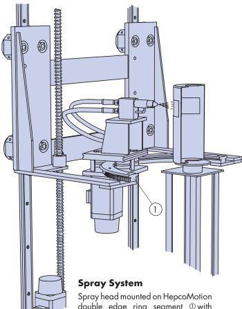
Spray head mounted on HepcoMotion double edge ring segment ① with external gear drive, tracks curvature of product.
