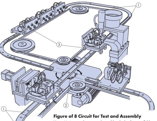
HepcoMotion track system ① enables hydraulic manifolds to be friction driven to a test station and then to subsequent assembly and unload stations or, if rejected, back to the load station. The unique ability of the Hepco System to traverse from one slide to another, enables a turntable to be designed at the crossover junction using a HepcoMotion ring disc ② to provide rotary movement. Bogie carriages ③ allow S bends to be traversed.
