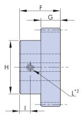
Pinion shown is BK type bore > 8mm
