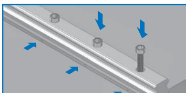
Step 3: Fasten bolts temporarily
