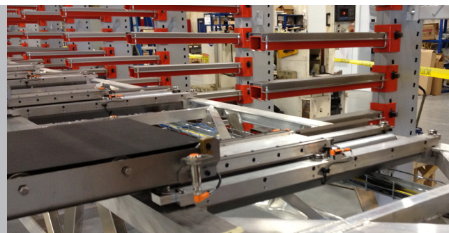
Studded DualVee guide wheels and track mounted to conveyor frames provide motion for a double extending telescopic solution.
