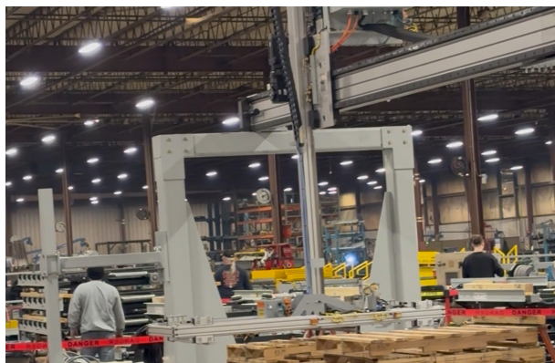
Lower-profile gantry system designed for efficient pallet transfer in a high-throughput corrugated conveyor application.
