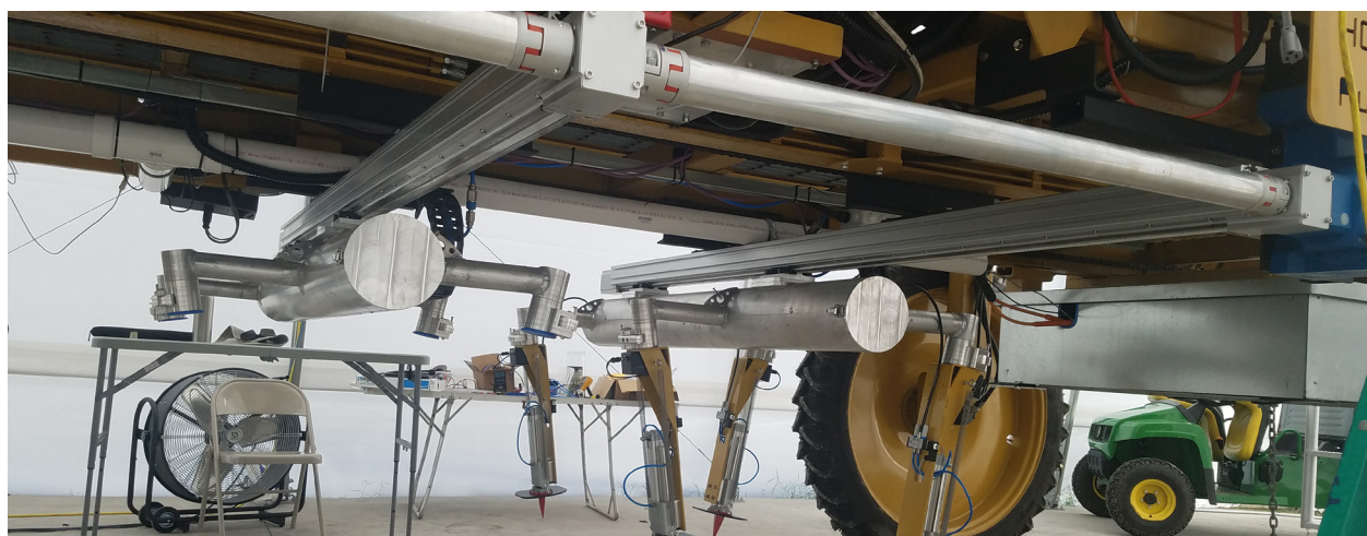
Strawberry picker undercarriage with daisy-chained actuators for carrying the individual robotic elements.
